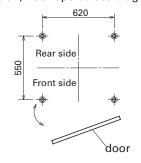
Anchor bolt (option)  $(4-M12 \times 160 \times 50)$
