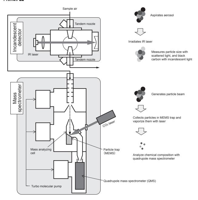
Aerosol analyzer consists of an incandescent detector and a mass spectrometer.
