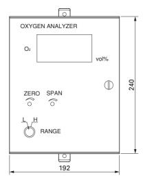
\* Change switch is not attached in the case of a single range.
