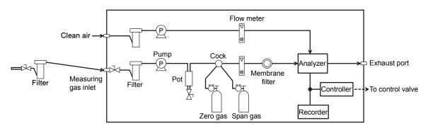
Note) This is the example of sampling which dose not contain water in the measuring gas.
