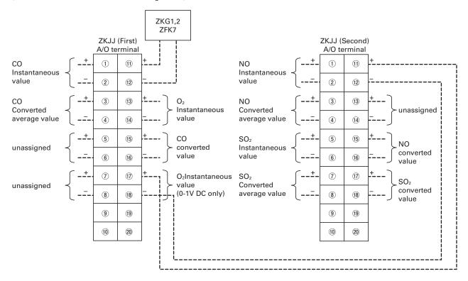
Measurment of NO/SO $_2$ /CO $_2$ CO/O $_2$  sensor [Example connection] (with converted value and converted average value)
